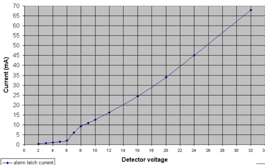
**Fig. 4 Alarm Load Presented to the Controller**
