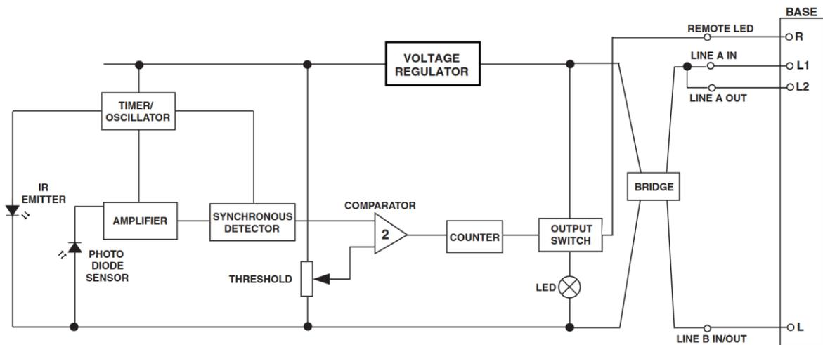
**Fig. 2 Block Schematic of Detector**
