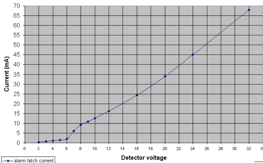
**Fig. 4 Alarm Load Presented to the Controller**
