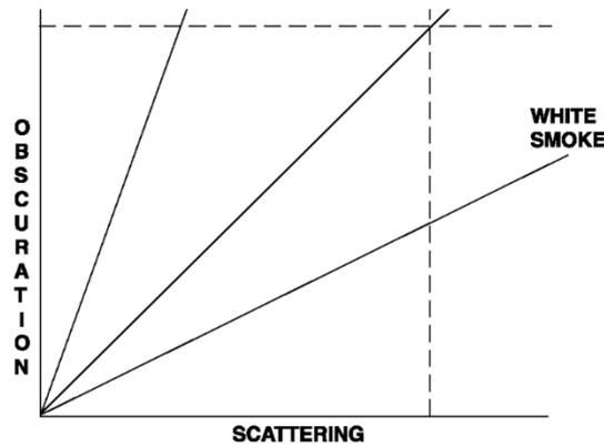
**Fig. 5 Response Threshold vs Smoke Colour**
