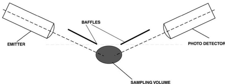
**Fig. 1 Optical System Schematic**
