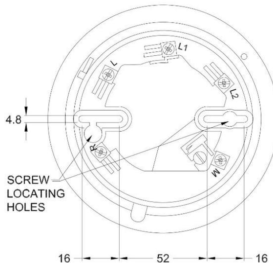
**WIRING**—Collective Cables are connected to base terminals L (-In/Out) and L1 (+ In) and L2 (+Out) for Collective systems. A Remote Indicator may be connected between positive L1 (+) and R (-).
