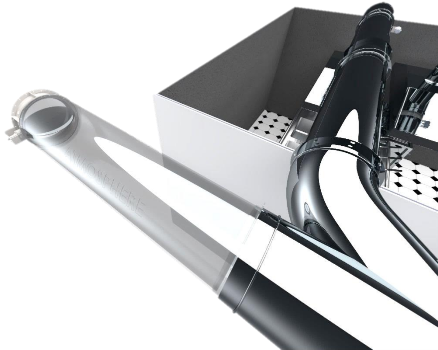
Fig. 1.4. Opened Air Damper To The Amosphere
