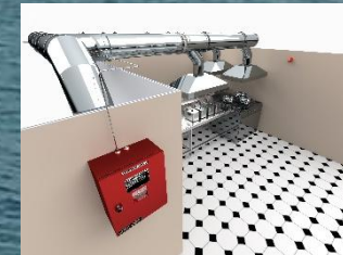
GALLEY DUCT CO 2 SYSTEM
